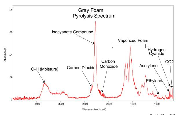
Figure 13. Infrared spectrum of gray foam pyrolysis with gases labeled. The more oxygen starved the combustion the more the final products will be similar to the pyrolysis products.
