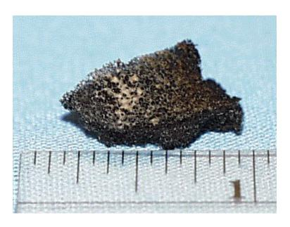
Figure 7. Sample 0310027-02 piece1 foam with adhesive.
