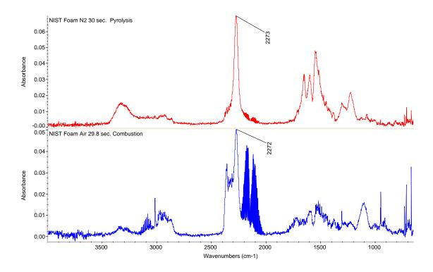
Figure 2. Infrared spectrum of foam pyrolysis gases (top) and combustion gases (bottom). The dominate peak in each spectrum is the peak at ~2270 cm<sup>-1</sup>). This peak most closely matches isocyanate compounds (see figure 3). The related isocyanide compounds are not a good match (see figure 4) because their absorbance is too far from 2270 cm<sup>-1</sup>.
