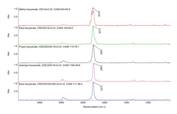
Figure 3. Infrared spectra of selected isocyanate compounds all with absorbances in the 2270 +/- 9 cm<sup>-1</sup> range. These are some of the most likely compounds to match the 2270 cm<sup>-1</sup> peak in the pyrolysis and combustion spectra (Figure 2.).
