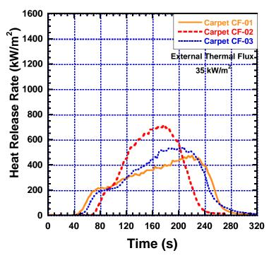
Figure D-22. Heat Release Rate versus Time for Carpet Sample Exposed to 35 kW/m² of External Heat Flux (CF). Samples are CF-01, CF-02, and CF-03.
