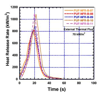
Figure D-13. Heat Release Rate versus Time for Polyurethane Foam Exposed to 70 kW/m<sup>2</sup> of External Heat Flux (PUF-NFR-B). Samples PUF-NFR-B-07, PUF-NFR-B-08, PUF-NFR-B-10, and PUF-NFR-B-11.
