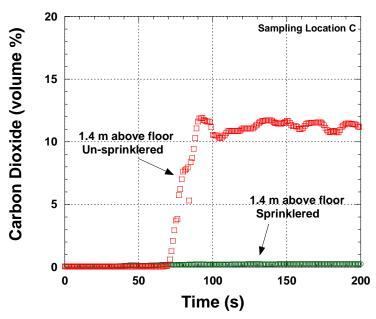
Figure G-12. Carbon dioxide volume fraction versus time for unsprinklered and sprinklered mockup test. Gas sampling probe positioned on main floor (Location C) at 1.4 m (4.5 ft) above floor.
