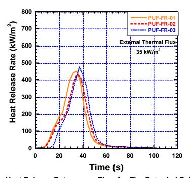
Figure D-15. Heat Release Rate versus Time for Fire Retarded Polyurethane Foam Exposed to 35 kW/m<sup>2</sup> of External Heat Flux. Samples PUF-FR-01, PUF-FR-02, and PUF-FR-03.
