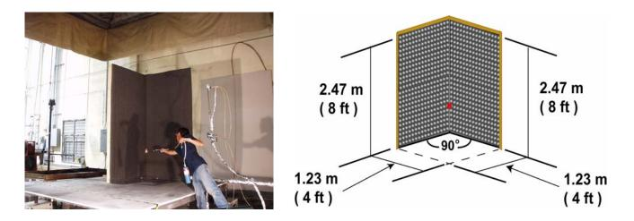
Figure E-2. Photograph and Dimensioned Diagram of Internal Corner
