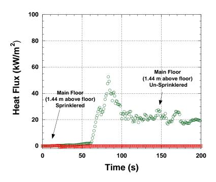
Figure G-18. Heat Fluxes versus Time for Unsprinklered and Sprinklered Mockup. Gauges positioned facing ceiling (1.44 m above floor) at location C.
