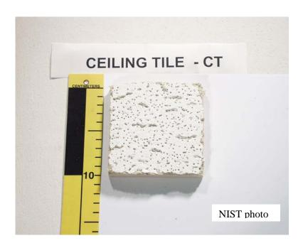
Figure D-16. Photograph of Acoustical Tile Showing Factory Painted Surface.
