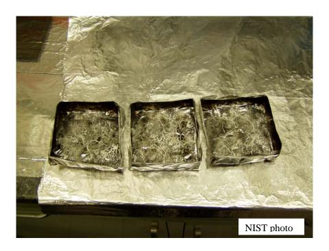
Figure D-4. Burn Residue of Polyurethane Foam after Cone Calorimeter Test.
