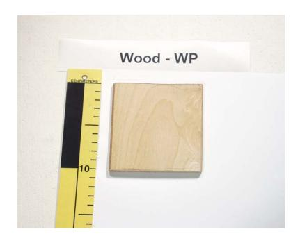
Figure D-18. Photograph of Wood Panel Sample Showing Veneer Surface.
