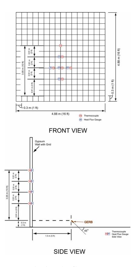
Figure F-7. Instrumentation Diagram for a Single Gerb at 45 degrees and in a Plane Perpendicular to Wall.
