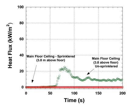
Figure G-21. Radiation Fluxes versus Time for Unsprinklered and Sprinklered Mockup. Gauges positioned flush with ceiling, facing down (3.8 m above floor) at location D.
