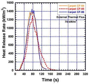
Figure D-23. Heat Release Rate versus Time for Carpet Sample Exposed to 70 kW/m² of External Heat Flux (CF). Samples are CF-04, CF-05, and CF-06.
