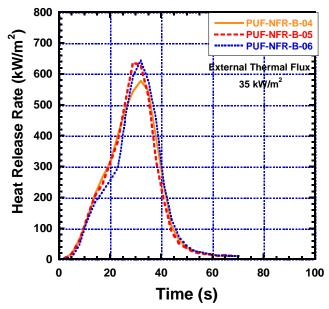
Figure D-10. Heat Release Rate versus Time for Polyurethane Foam Exposed to 35 kW/m<sup>2</sup> of External Heat Flux (PUF-NFR-B). Samples PUF-NFR-B-04, PUF-NFR-B-05, and PUF-NFR-B-06.
