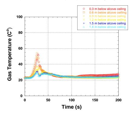
Figure G-6. Temperatures versus Time for Sprinklered Mockup Test. Thermocouples positioned in Alcove (A-SR) on wall (stage-right).
