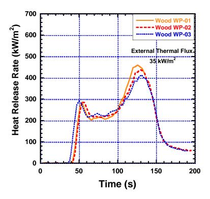
Figure D-19. Heat Release Rate versus Time for Wood Paneling Exposed to 35 kW/m<sup>2</sup> of External Heat Flux (WP). Samples are WP-01, WP-02, and WP-03.
