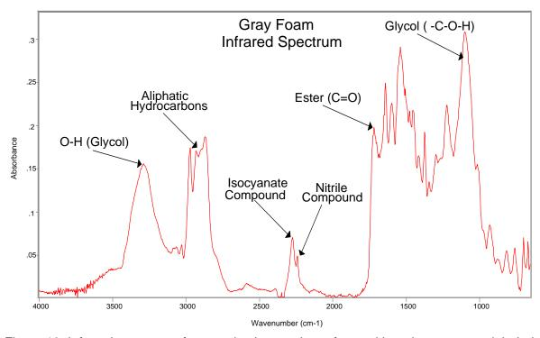
Figure 19. Infrared spectrum of gray polyether urethane foam with major structures labeled.
