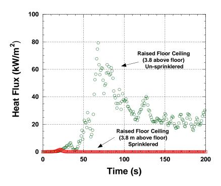
Figure G-22. Radiation Fluxes versus Time for Unsprinklered and Sprinklered Mockup. Gauges positioned flush with ceiling, facing down (3.8 m above floor) at location B.
