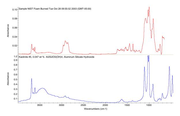
Figure 10. Infrared spectrum of sample foam adhesive (top), Best library match of the mineral filler kaolinite  $Al_2Si_2O_5(OH)_4$ , (bottom).
