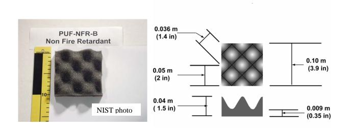
Figure D-6. Photograph and Dimensioned Diagram of Non Fire Retardant Foam Lot B (PUF-NFR-B).
