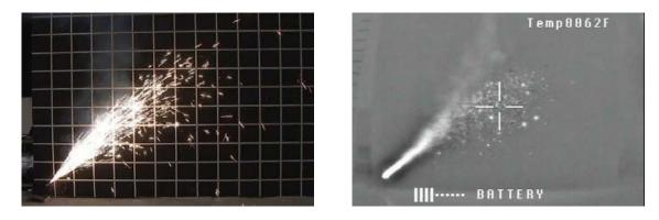
Figure F-9. Standard Video and Infrared Video Images of Gerb Discharge at 2 s.
