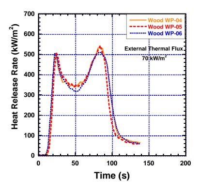
Figure D-20. Heat Release Rate versus Time for Wood Paneling Exposed to 70 kW/m<sup>2</sup> of External Heat Flux (WP). Samples are WP-04, WP-05, and WP-06.
