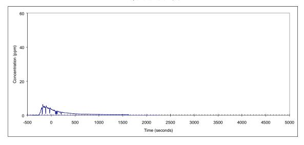
Figure J-4. Hydrogen cyanide response from mini gas analyzer located at position 1.
