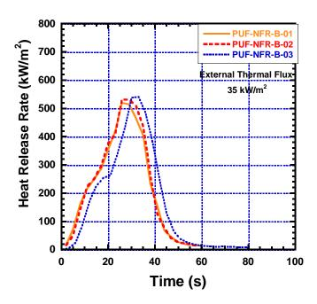
Figure D-9. Heat Release Rate versus Time for Polyurethane Foam Exposed to 35 kW/m<sup>2</sup> of External Heat Flux (PUF-NFR-B). Samples PUF-NFR-B-01, PUF-NFR-B-02, and PUF-NFR-B-03.
