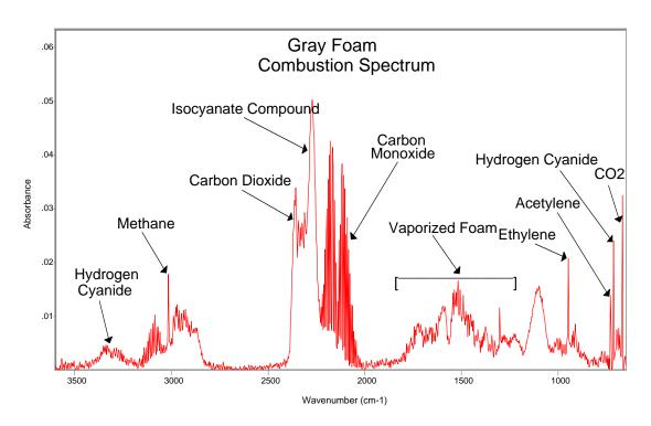
Figure 17. Infrared spectrum of gray foam combustion with combustion gases labeled
