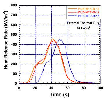
Figure D-8. Heat Release Rate versus Time for Polyurethane Foam Exposed to 20 kW/m<sup>2</sup> of External Heat Flux (PUF-NFR-B). Samples PUF-NFR-B-13, PUF-NFR-B-14, and PUF-NFR-B-15.
