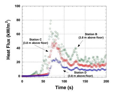
Figure G-15. Radiation fluxes versus time for unsprinklered mockup test. Gauges positioned flush with ceiling (3.8 m above floor) at locations B, C, and D.
