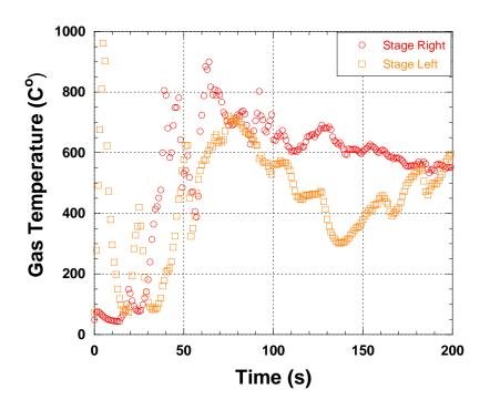
Figure G-3. Temperatures versus Time for Unsprinklered Mockup Test. Thermocouples positioned on right and left side of alcove opening 1.8 m (5.t ft) above platform floor at ignition points.
