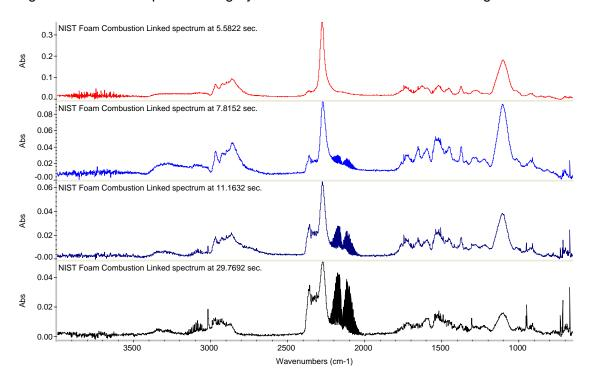
Figure 18. Infrared spectrum of foam combustion progression. Note the growth of the carbon monoxide peak (centered at 2150 cm<sup>-1</sup>) as the combustion progresses from 5 to 30 seconds. The isocyanate compound peak (~2270 cm<sup>-1</sup>) dominates each spectrum. The polypropylene peak (~1100 cm<sup>-1</sup>) is decreasing showing that the oily polypropylene glycol compound is being consumed as the combustion progresses.
