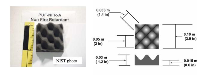
Figure D-5. Photograph and Dimensioned Diagram of Non Fire Retardant Foam Lot A (PUF-NFR-A).
