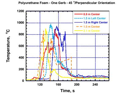
Figure F-16a. Temperatures versus Time for Single Gerb Discharged at 45 Degrees in Plane Perpendicular to Wall.
