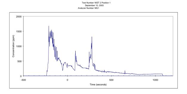
Figure J-6. Hydrogen cyanide response from mini gas 1 located at position 1
