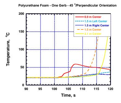
Figure F-16b. Temperatures versus Time for Single Gerb Discharged at 45 Degrees in Plane Perpendicular to Wall.
