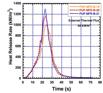
Figure D-12. Heat Release Rate versus Time for Polyurethane Foam Exposed to 60 kW/m<sup>2</sup> of External Heat Flux (PUF-NFR-B). Samples PUF-NFR-B-19, PUF-NFR-B-20, and PUF-NFR-B-21.
