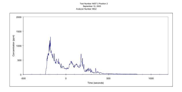
Figure J-7. Hydrogen cyanide response from mini gas 2 located at position 2.
