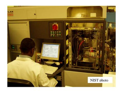
Figure D-1. Cone Calorimeter – Test Chamber (right side), computer display (center), and gas analyzers (left side).
