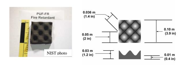
Figure D-14. Photograph and Dimensioned Diagram of Fire Retardant Foam (PUF-FR).
