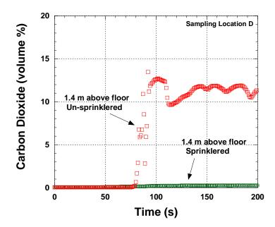
Figure G-13. Carbon dioxide volume fraction versus time for unsprinklered and sprinklered mockup test. Gas sampling probe positioned on main floor (Location D) at 1.4 m (4.5 ft) above floor.
