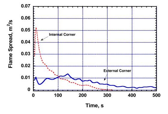
Figure E-10. Flame spread across foam covered wall panel (m<sup>2</sup>/s).
