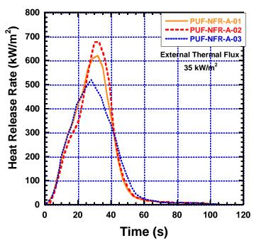
Figure D-7. Heat Release Rate versus Time for Polyurethane Foam Exposed to 35 kW/m<sup>2</sup> of External Heat Flux. Samples PUF-NFR-A-01, PUF-NFR-A-02, and PUF-NFR-A-03.
