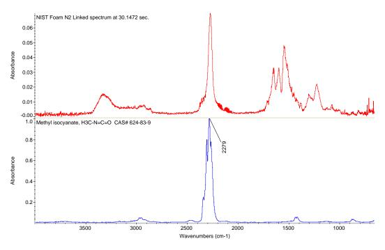
Figure 12. Infrared spectrum of sample pyrolized foam (top). Best library match is methyl isocyanate (peak ~2270 cm<sup>-1</sup>). This is a match to a class of isocyanate compounds. Methyl, Propyl, and even Butyl isocyanate have spectra that cannot be distinguished at this resolution.
