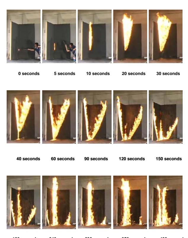
180 seconds 240 seconds 290 seconds 350 seconds 400 seconds Figure E-8. Flame spread over polyurethane foam covered panels, internal corner configuration.
