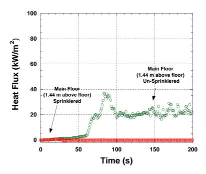
Figure G-16. Heat Fluxes versus Time for Unsprinklered and Sprinklered Mockup. Gauges positioned facing alcove (1.44 m above floor) at location C.
