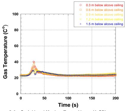
Figure G-8. Sprinklered Mockup Test. Alcove (A-SB) on rear wall.
