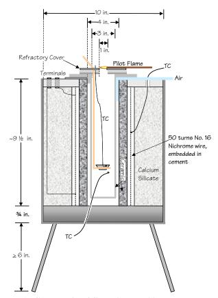
Figure 1. Schematic of SwRI's Hot-Air Furnace.
