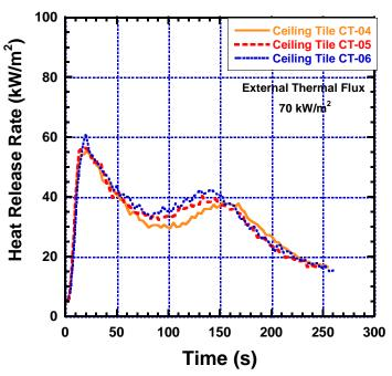
Figure D-17. Heat Release Rate versus Time for Ceiling Tile Exposed to 70 kW/m<sup>2</sup> of External Heat Flux. Samples are CT-04, CT-05, and CT06.
