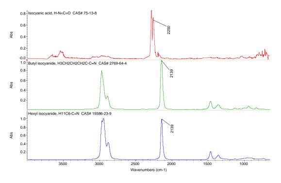
Figure 4. Infrared spectra of selected isocyanide compounds. These have a slightly different structure than the isocyanate compounds in Figure 3. These do not match the 2270 cm<sup>-1</sup> peak in the pyrolysis and combustion spectra (Figure 2.).
