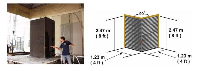
Figure E-1. Photograph and Dimensioned Diagram of External Corner
