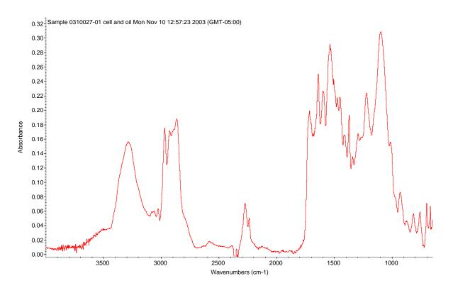
Figure 3. Infrared spectrum of sample unburned gray foam.
