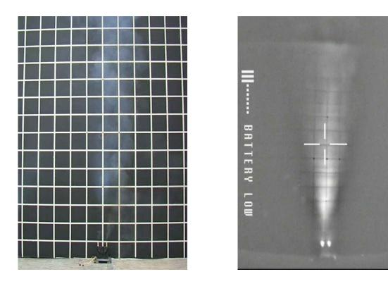
Figure F-22. Standard Video and Infrared Video Images of Gerb Discharge at 16 seconds.
