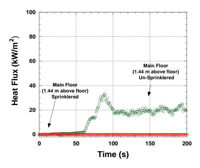
Figure G-17. Heat Fluxes versus Time for Unsprinklered and Sprinklered Mockup. Gauges positioned facing alcove (1.44 m above floor) at location D.
