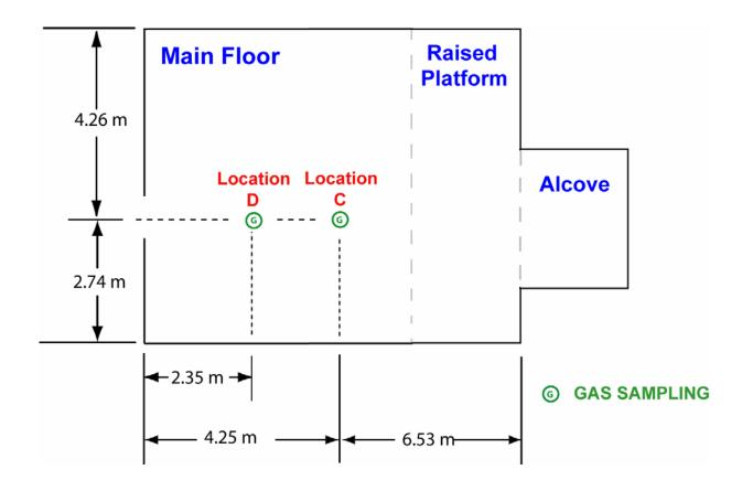
Figure G-11. Schematic floor plan with gas sampling locations.
