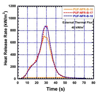
Figure D-11. Heat Release Rate versus Time for Polyurethane Foam Exposed to 40 kW/m<sup>2</sup> of External Heat Flux (PUF-NFR-B). Samples PUF-NFR-B-16, PUF-NFR-B-17, and PUF-NFR-B-18.
